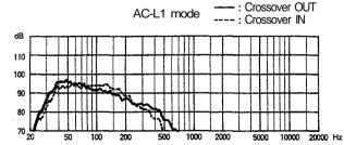
General frequency response (1W/1m, at 300Hz of the SR-F1B) SR-L1B+AC-L1, SR-F1B+AC-F1 AC-L1: Crossover OUT
