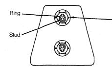
Fitting metal supplied with the SR-F1B 32202 Ring/Stud Pan Fitting (Aeroquip made)
