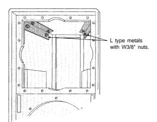
L type metals with W3/8" nuts are provided at four corners inside the enclosure as shown in the figure. Nuts are located just at back side of the fixing holes of the enclosure. Utilize these fixing holes according to installation places of the speaker. Refer to appearance diagram on the fixing holes.
