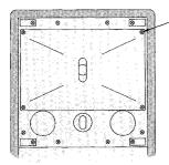
Fixing screws for the baffle (14 positions)
