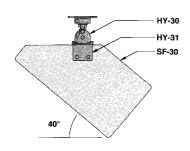
T-nuts for ceiling suspension are provided on rear slant and both sides of enclosure, permitting the SF-30 to be readily suspended from the ceiling when used with the optional brackets, HY-30 and HY-31. (Bolts to fix the brackets to the speaker are supplied with the HY-30.) The angle is adjustable 360 degrees horizontal, and  $\pm$ 10 degrees vertical from the angle in the figure. Refer to the instruction manual of the HY-30 for details.
