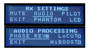
OFF. Navigate to each option by rotating the "Jog-Wheel" and press to check the box for each option when it is underlined.
