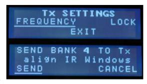
seconds. All frequencies in the bank selected will be transferred to the transmitter and its current frequency will be set to match the receiver's current frequency. The receiver will return to its main display.
