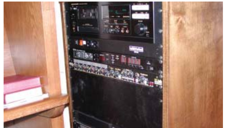
▲ A Marantz 502 provides the capability to record the service straight out of the Whirlwind Mix 6F stereo mixer.
