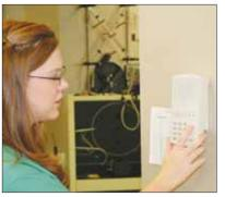
A staff member at the rehabilitation center demonstrates the facility's new intercom system. Use of the IP intercom products occupy minimal network bandwidth (130kbps maximum) for station-to-station calls and can be controlled and monitored through software or a Web browser.
