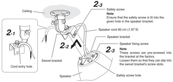
**Step 3.** Connect the 60 cm (1.97 ft) speaker cord to the routed speaker cable.
