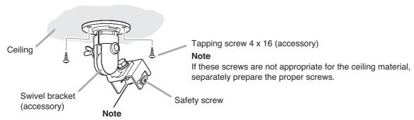
Loosen the safety screw until it's tip does not stick out from the bracket surface. If the screw tip sticks out, this obstructs the insertion of the speaker bracket in Step 2.
