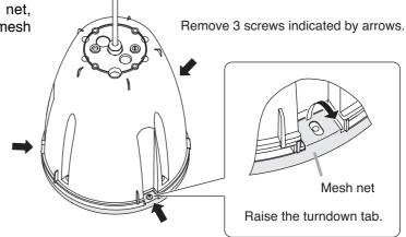
**Step 3.** Clean the speaker cover and mesh net. Wipe with a soft cloth damped in a detergent.
