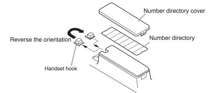
Step 3. After replacing the directory on the station, hook the directory cover's forward tab and push on the upper part of the directory cover.
