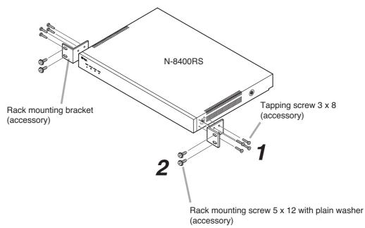
Step 1. Install the rack-mounting bracket to the N-8400RS.
