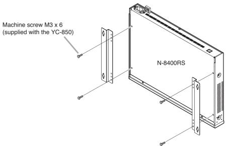
Step 2. Mount the N-8400RS on the wall.
