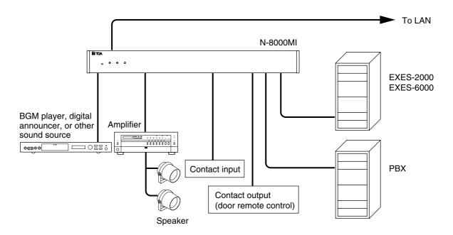
Having 2 channels each for audio input and output, and 16 contacts each for control input and output, the N-8000MI performs the following interface functions\*.
