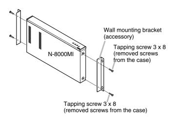
Step 2. Mount the N-8000MI on the wall.
