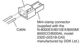
**Step 2.** With a pair of pliers, lightly pinch the mini-clamp cover and, after ensuring that the cable is securely inserted, firmly squeeze on the cover.
