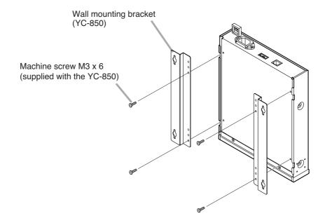
Step 2. Mount the N-8000AL on the wall.
