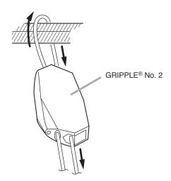
Step 3. Adjust the length of the hanging wire for the optimum speaker mounting height.
