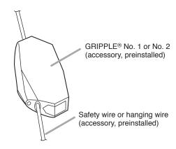
**Step 2.** Pass the hanging wire over the ceiling anchor point such as beam or purlin, then pass it through the other hole in the GRIPPLE® No. 2.
