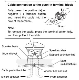
**Step 1.** Connect the speaker cables that have been run through the cable protective tube to the push-in terminals inside the speaker base.
