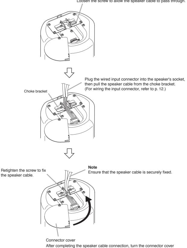
in the direction indicated by the arrow, and fix the cover with 2 screws.
