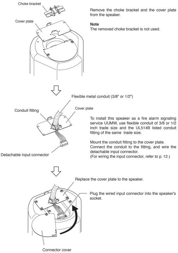
After completing the speaker cable connection, turn the connector cover in the direction indicated by the arrow, and fix the cover with 2 screws.
