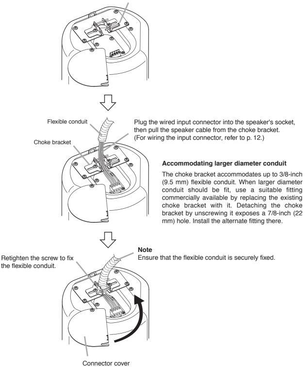
After completing the speaker cable connection, turn the connector cover in the direction indicated by the arrow, and fix the cover with 2 screws.
