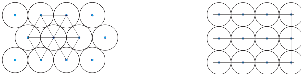
Figure 6-2 Speaker coverage with no overlap: hexagonal (left), square (right)
