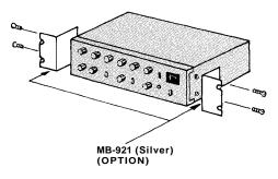
Fix the MB-921 with attached 4 screws. The length of the screws should not exceed 12mm (1/2 inches).
