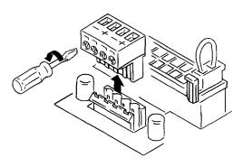
2-3. Insert the stripped cable ends into the input connector, and tighten the connector screws.
