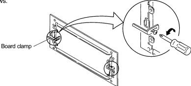
1-3. Place the Adapter Panel inside the opening, and set the panel to the desired position using the positioning tabs.
