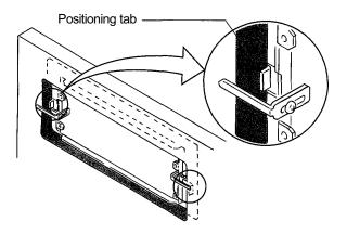
1-4. Clamp the wall or ceiling panel using the two board clamps, and secure with the clamp screws.
