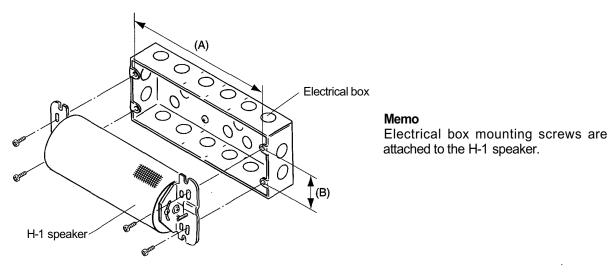
**Note:** The distance between the wall or ceiling surface and the box bottom surface must be 45 mm or more. When using the Raco 953 electrical box, be careful in installation because it is shallow.
