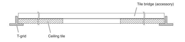
Place the supplied tile bridge on the 2-foot tile as shown at right.
