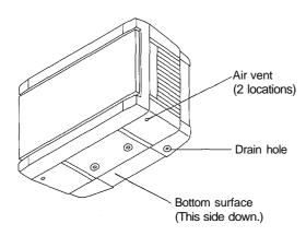
(2)As shown in the figure below, the speaker can be positioned at any angle from 0° (horizontal) to a 45° downward angle. As this mounting range permits free drainage of rainwater from the inside of the speaker, do not exceed this range, nor direct the speaker upward.
