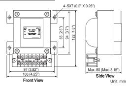
**Matching Transformer**Designed for use with the DA-500F-HL Multi-Channel Power Amplifier (option), the MT-251H electrically isolates the high-impedance speaker lines from the amplifier.
