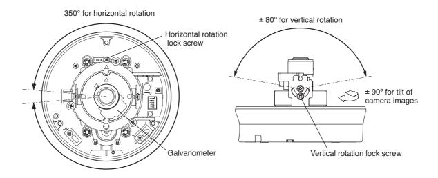
After angle adjustment completion, tighten both rotation lock screws.
