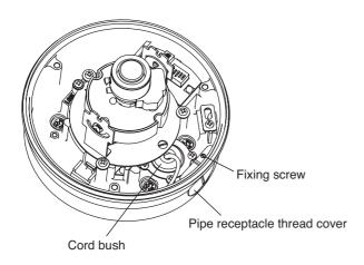
2. Push in the cord bush attached to the camera unit from the back to pull out from the case. Run the cable and lead it out from the camera pipe receptacle thread hole.
