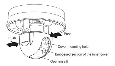
1-2. After attaching the inner cover, check to be sure that inner cover is securely fitted to the camera unit by pulling down the sections indicated by arrows tightly.
