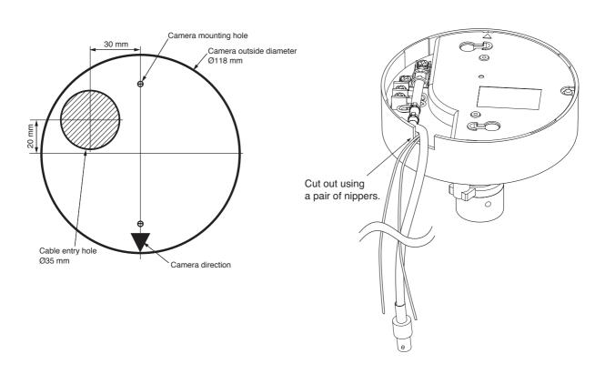
2. Mount the camera to the ceiling or wall using 2 mounting screws.
