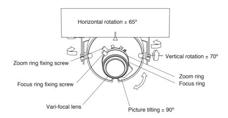
5. Adjust the angle of view with the Zoom ring and adjust the focus with the Focus ring for the best possible picture reproduction. After lens adjustment completion, tighten both the Zoom ring fixing screw and the Focus ring fixing screw.
