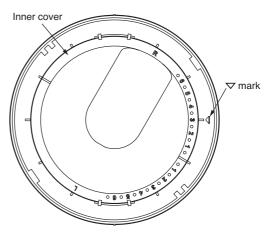
Rotate the inner cover to the "R" range, and align the √mark with scale indicator "3."
