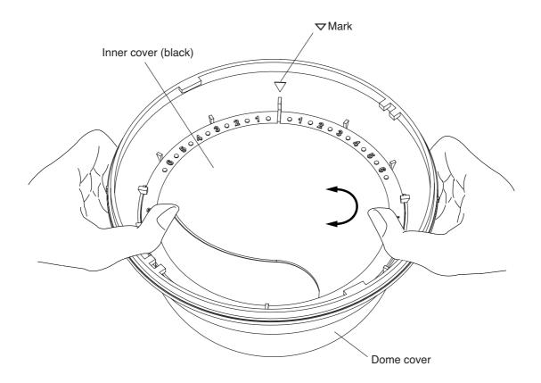
3-2. Attach the dome cover to the camera by aligning the dome cover's alignment mark with the camera's △ mark and then rotating the cover clockwise.
