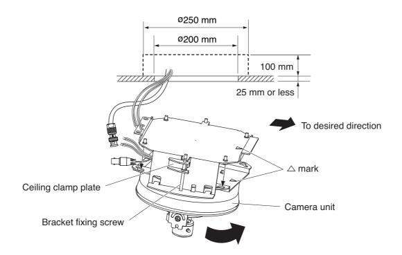
6. Install the camera to the flush ceiling mounting bracket.
