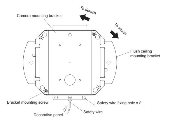
3. Install the camera to the removed camera mounting bracket using the supplied M4 x 10 camera mounting screws.
