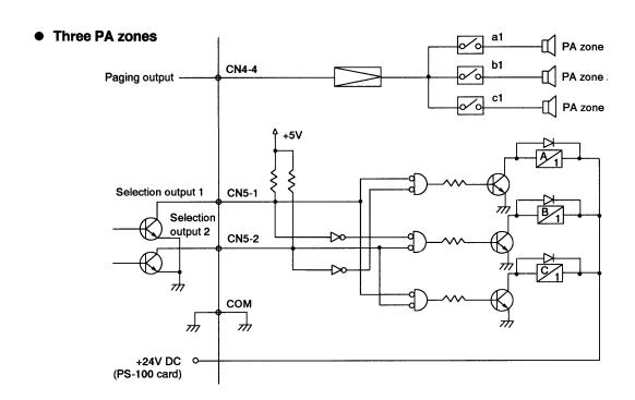
[Note]: The PS-100'S power voltage (24V DC) fluctuates from 22V to 30V. When using the PS-100 to supply power to the relay, therefore, care must be given to the relay's operating voltage.
