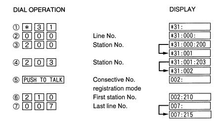
(3) Register connected tie-line system control stations and sub-stations.
