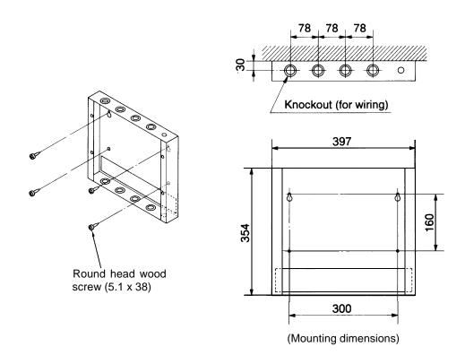
② After removing the CK-100's front panel, mount the unit on the Wall Mounting Frame.
