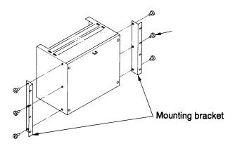
② Mount the unit in a standard equipment rack.
