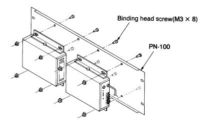
3 Mount the PN-100 in a standard equipment rack.
