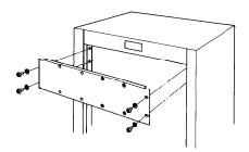
[Note] : Perform terminal wiring before mounting.
