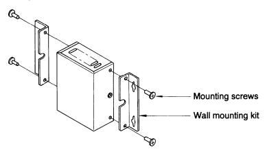
② Mount the unit on the wall using the supplied wood screws.
