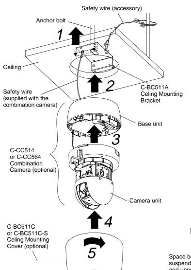
Be sure to carefully read the installation manual supplied with the camera.
