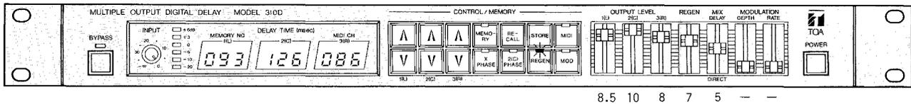
**5. FLANGING EFFECT** By mixing the delayed signal of 2(C) with the direct signal, a main flanging effect can be obtained, and a side flanging effect results from a cross-phased 1(L) and 3(R). The delay time of 2(C) and the 2(C) phase switch both play a main role in determining the timbre. Both 1(L) and 3(R) give a sense of sound "spreading". Set the cross phase switch to OFF for monoaural output.
