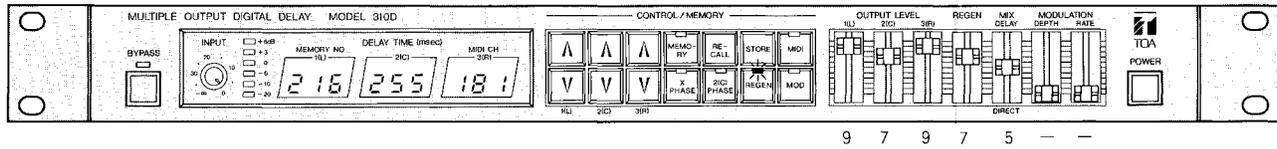
**2. ECHO 2** An echo having delay times much different from each other. Placing the Regeneration (feedback) switch in the off position produces gated echo-like sounds.
